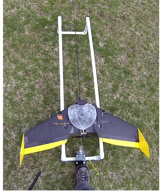
Fig. 5: Aircraft hardware in the field. We use a small catapult for consistent launches near obstacles.
