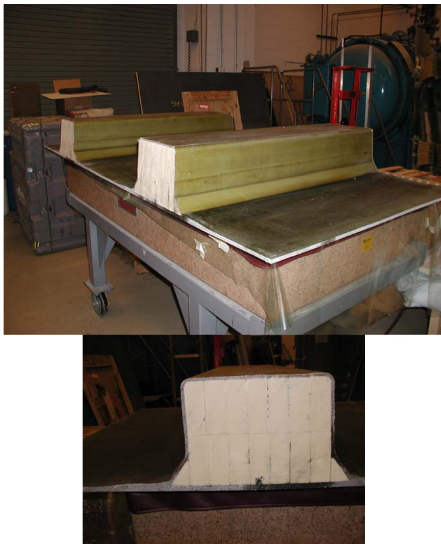
Figure 178. Hat-stiffened structure showing the final hat-stiffened structure and a close-up of the hat-stiffened area.
