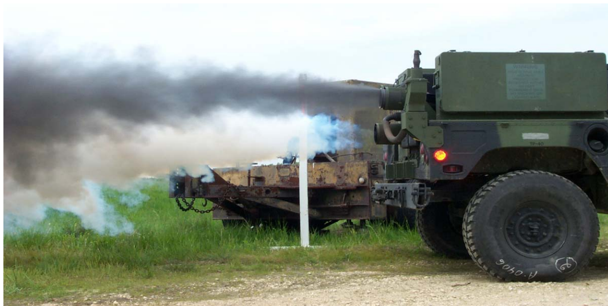
Figure 1. FO and graphite smoke generation from one vehicle; FO smoke is white and graphite flake smoke is black.
