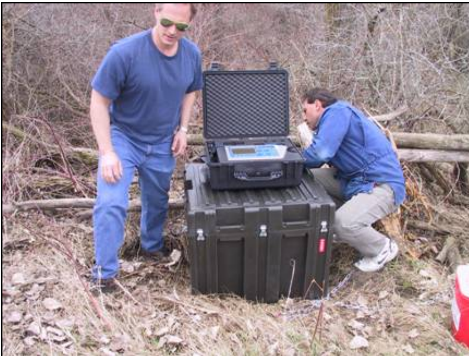
Figure 13. Installing a noise monitor. The battery box is the large lower box while the recording instrumentation is contained in the upper box.
