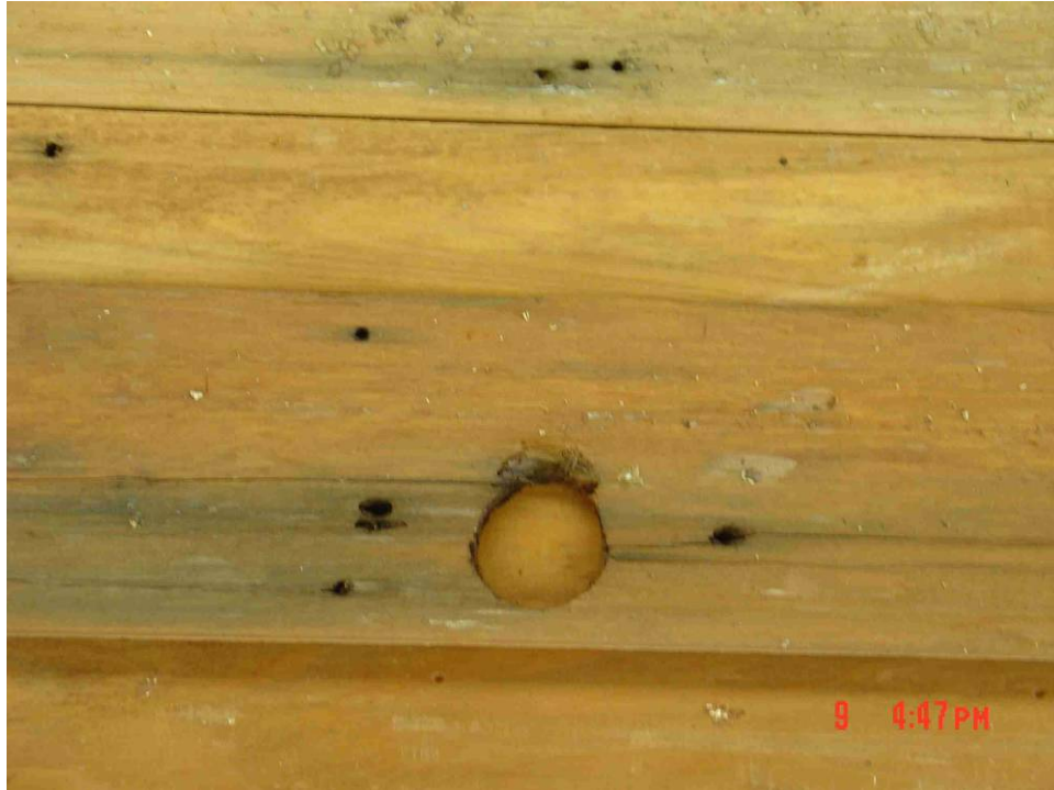
Figure 4.9. Utility holes found in a number of surveyed blank pieces.
