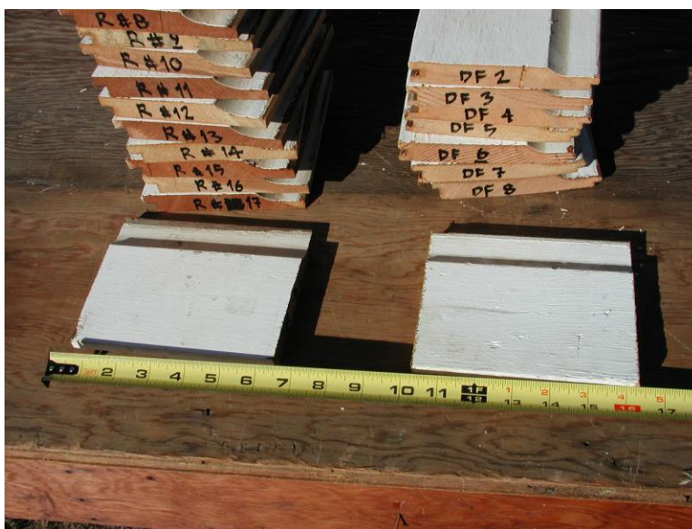
Figure 4.15. Siding samples awaiting lead penetration testing.
