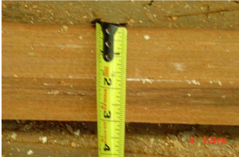
Figure 4.11. Produced blank that is too narrow.
