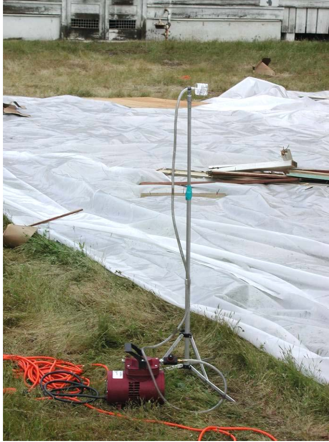
Figure 4.14. Ambient air monitoring device.
