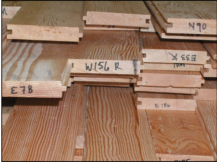
Figure 2.5. T&G flooring remanufactured from WWII-era barracks.
