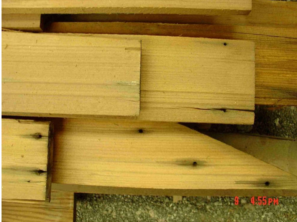
Figure 4.7. Examples of mitered cuts and end splits that would cause a loss of product yield.
