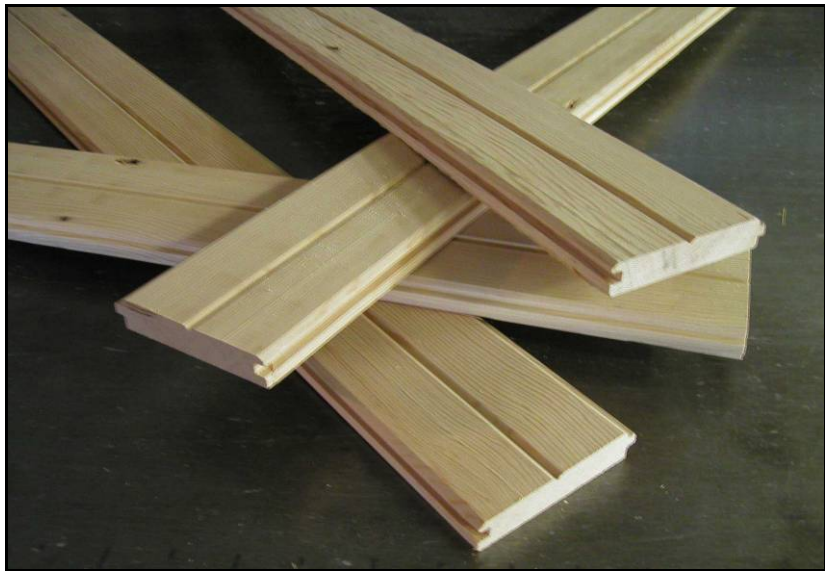
Figure 2.6. V-groove paneling remanufactured from WWII-era barrack.
