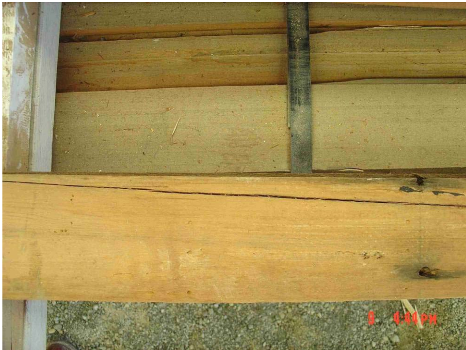
Figure 4.8. Lengthwise split as a defect that would cause a loss of product yield.
