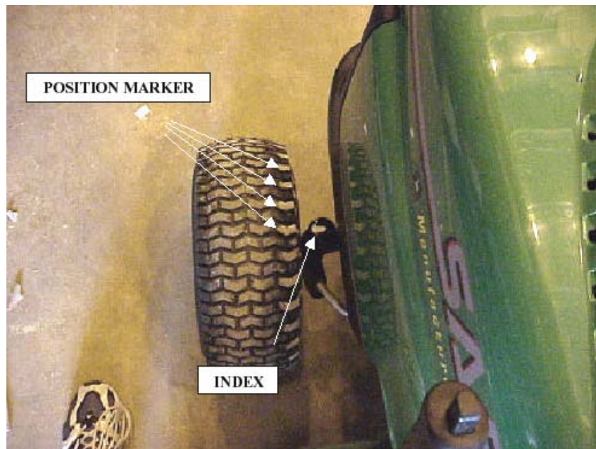
Figure 11. Marks on the front wheel for incremental positioning during each radar pass.
