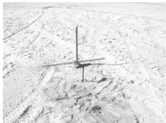
Figure 81 OSU/ESL soil probe inserted the ground to measure soil electrical property at different depths.
