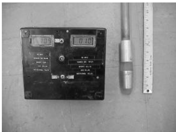
Figure 80 OSU/ESL soil probe for permittivity and conductivity measurement at 40 MHz and 60 MHz.
