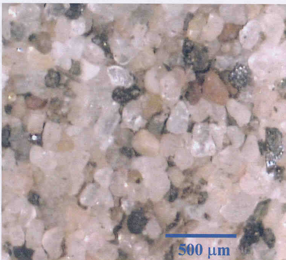
Figure 2. Milwaukee CDF sediment particles: 63-250 \mu\text{m} size fraction.
