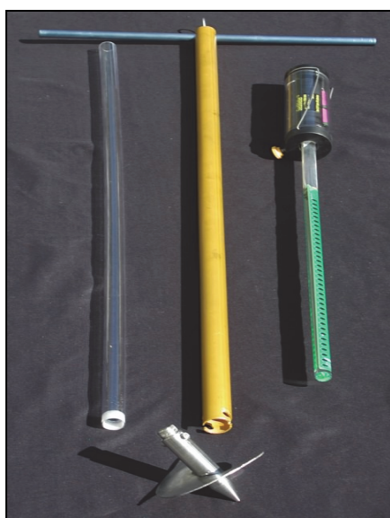
Figure 1. SediMeter (right) with the sampling tube (left) and auger system (middle). OBS detectors are contained within the green section on the instrument.
