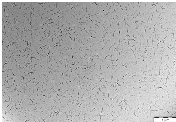
Figure 2. Transmission electron microscopy (TEM) image of CNCs isolated from microcrystalline cellulose (MCC) and deposited from a suspension in \text{CH}_2\text{Cl}_2 (0.03 mg/mL) onto a TEM grid and drying the sample at 70 °C for 3 h.
