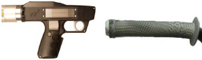
Figure 3: A grip with a handle that is at an angle offers better ergonomics to the user when compared to straight handles (right)
