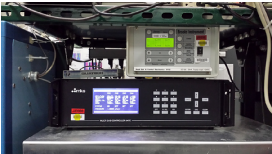
Figure A.3: User interface for the MKS propane controller (bottom) and low flow rate Brooks controllers (top)
