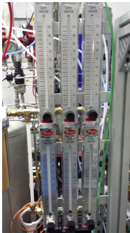
Figure A.6: Water needle valve flow controllers; Top bank (0-20 gallon per hour controllers): left and center - unused, right - rig wall cooling; Bottom bank (0-1 gallon per minute controllers): left - cooling for WSR bottom half, center - cooling for WSR top half, right - rig wall cooling
