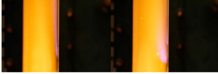
Figure 2.22: Secondary reactions occurring within a film cooling layer: slot injection (left); normal cylindrical hole injection followed by normal holes embeded within a trench (right) [14]
