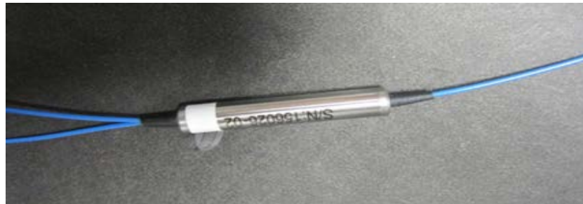
Figure 7: A Schematic and Picture of the Inline Fiber Splitter
