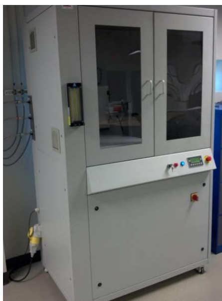
Figure 25. Plasmastream equipment for coating rigid substrates transferred to NDSU.
