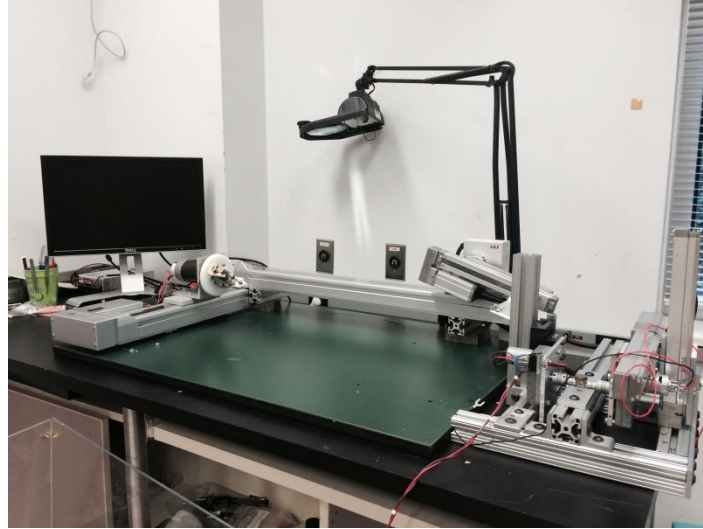
Figure 2. Automated winding and twisting machine designed for fabricating CNT fibers.
