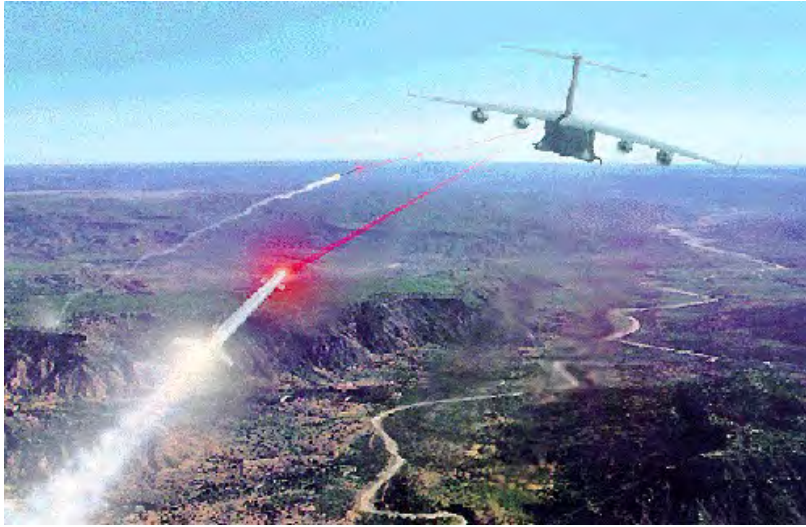
Figure 2-4. C-17 LAIRCM System
