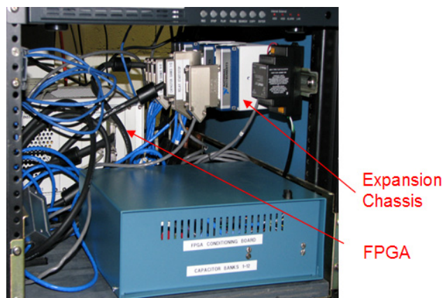
Figure 4. FPGA in PXI chassis and cRIO expansion chassis with expansion cards.
