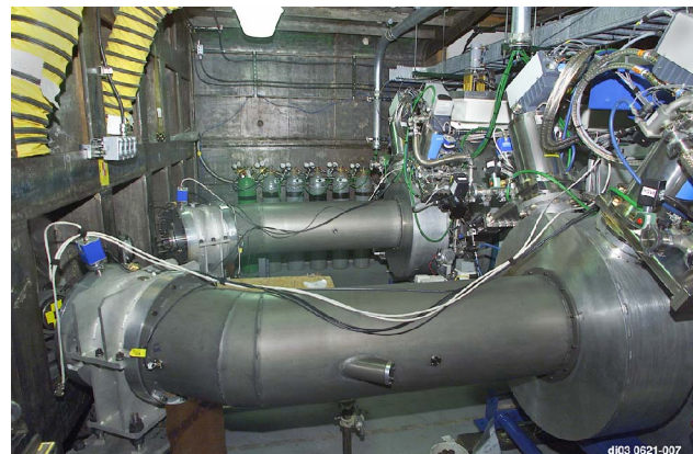
Figure 3. Cygnus installation at the U1a Complex. Top - Marx generators, Middle - Stalks removed from IVAs, and Bottom - VITLs (center) and angled Diodes (far left).
