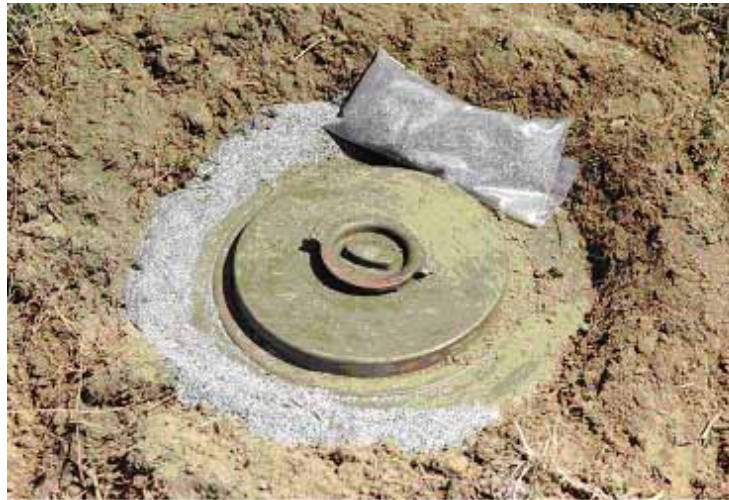
Figure 26. 0.9 kg (2 lb) of Thermite vs. M15 Anti-tank Mine
