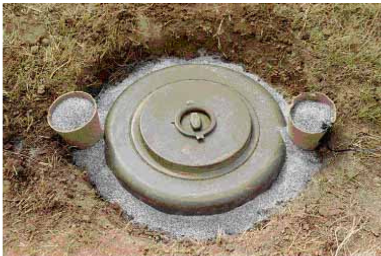
Figure 45. 3 kg ( 6 lb) of Thermite vs. an M15 Mine
