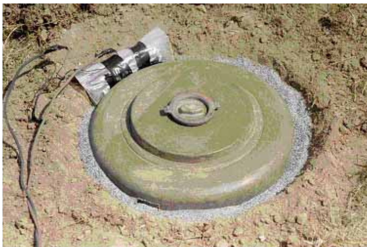
Figure 33. 0.9 kg (2 lb) of Thermite vs. M15 Anti-tank Mine
