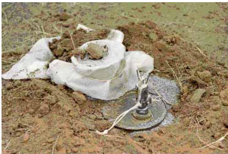
Figure 35. 0.9 kg (2 lb) of Thermite vs. M16A2 Anti-Personnel Mine
