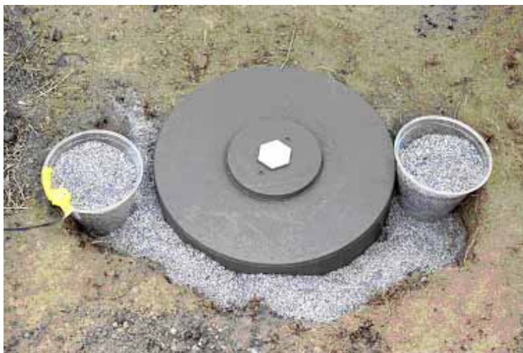
Figure 59. 2 kg (5 lb) of Thermite vs. M21 Mine
