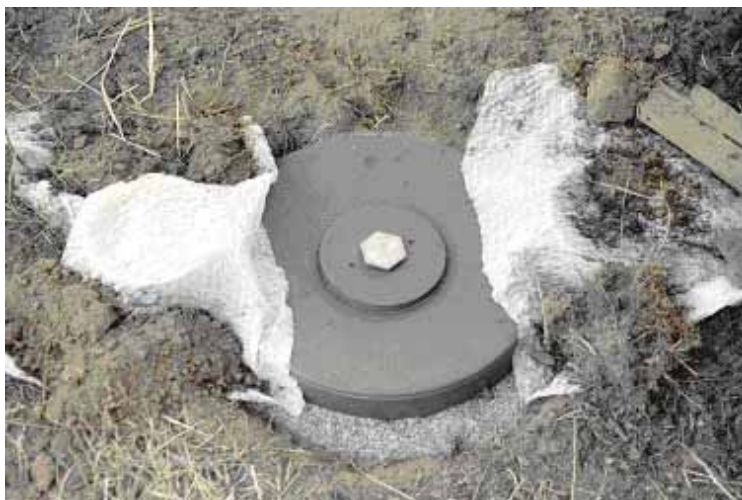
Figure 57. 2 kg (5 lb) of Thermite vs. M21 Mine
