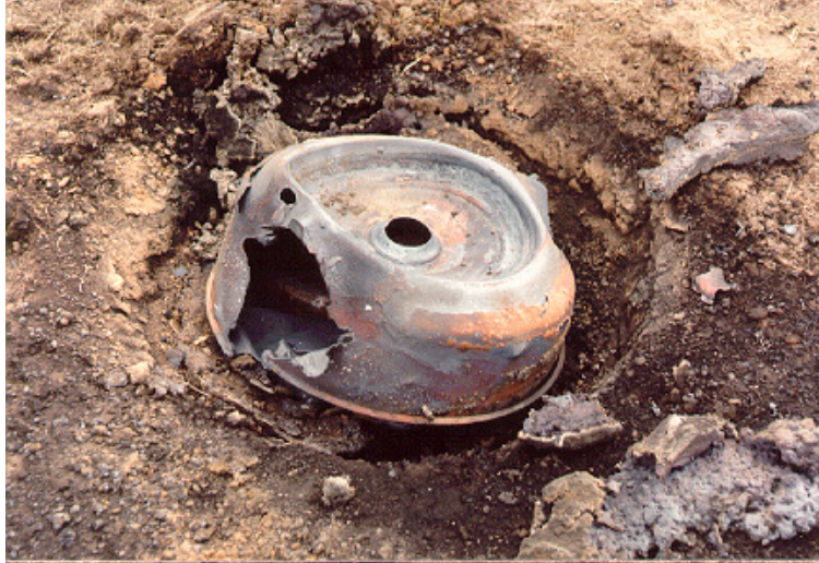
Figure 40. Burned out M15 mine case
