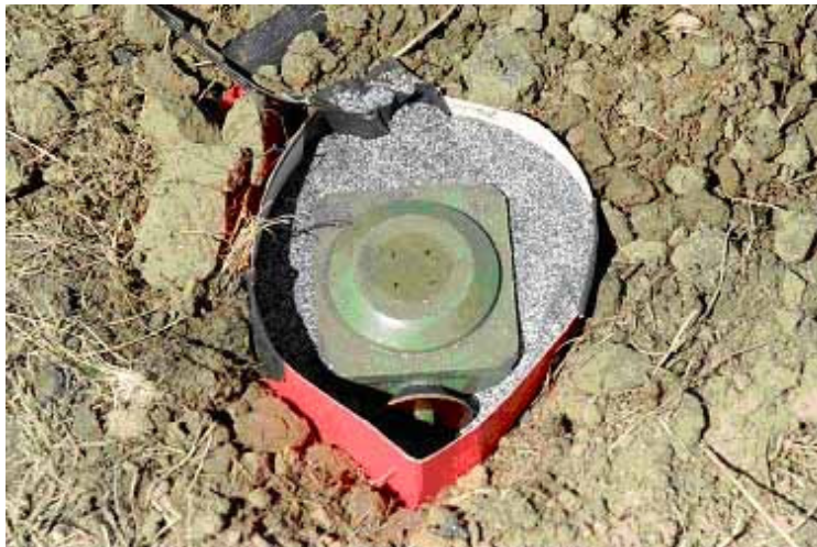
Figure 47. 0.5 kg (1 lb) of Thermite vs. PP-Mi-Na1 Mine
