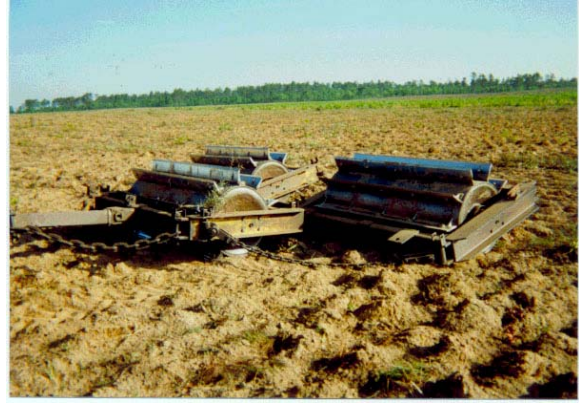
Figure 3-46. Roller Drum Choppers
