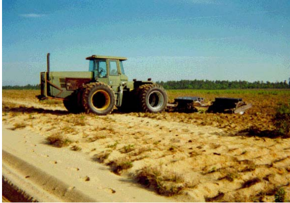
Figure 3-45. Typical Roller Drum Chopper Rig
