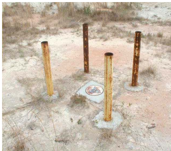
Figure 3-30. TA C-62 OB/OD Groundwater Monitoring Well MW94-62-03
