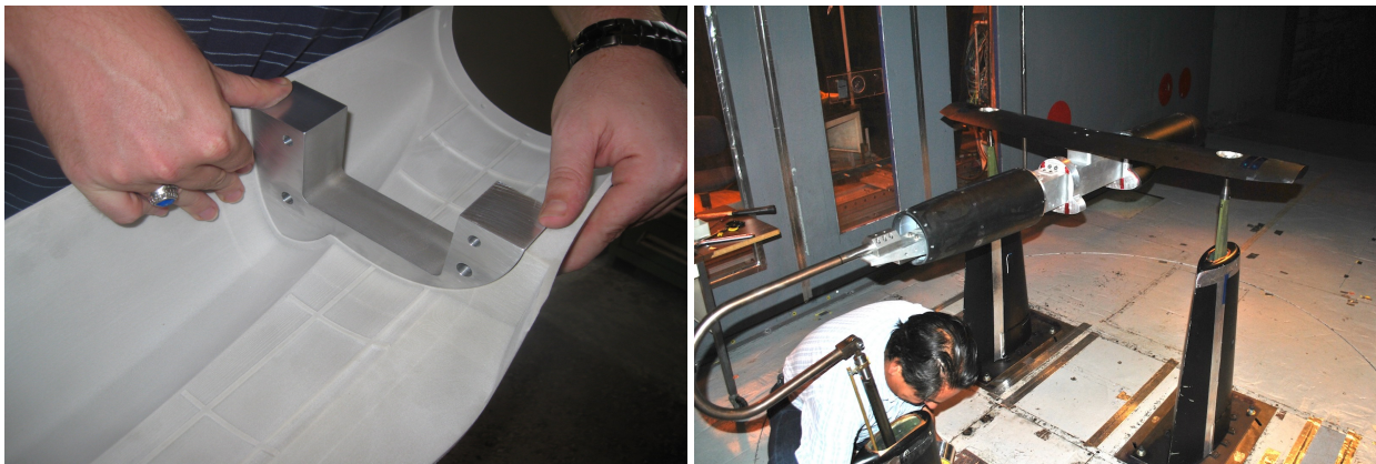
Figure 5: Example SLS fuselage panel fitted to rib (left). LCTR model being assembled in the wind tunnel (right) showing 4-in square aluminum tube strongback with portions of the fuselage fitted forward and aft of the wing.
