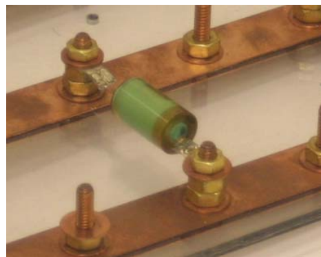
Figure 7. Diode packaged in similar but hollow hard epoxy barrel which was filled with silicone epoxy. Ring terminals were used to clamp the anode and cathode tabs onto quarter-inch brass bolts.
