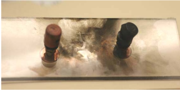
Figure 8. Clamp fixture which held failed diode. Lexan backing shows carbon debris. Clamp terminals had copper transfer from the anode and cathode tabs.
