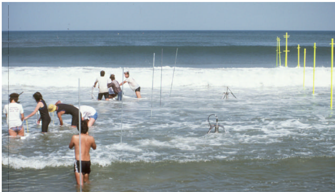
Figure 8. DUCK85 sediment transport experiment, directed by Dr. Nicholas Kraus (CHL). The researchers are tending sediment traps facing into the longshore current which is being measured by the two current meters located to their right. Further to the right, the line of photopoles was observed by movie cameras to measure wave conditions
