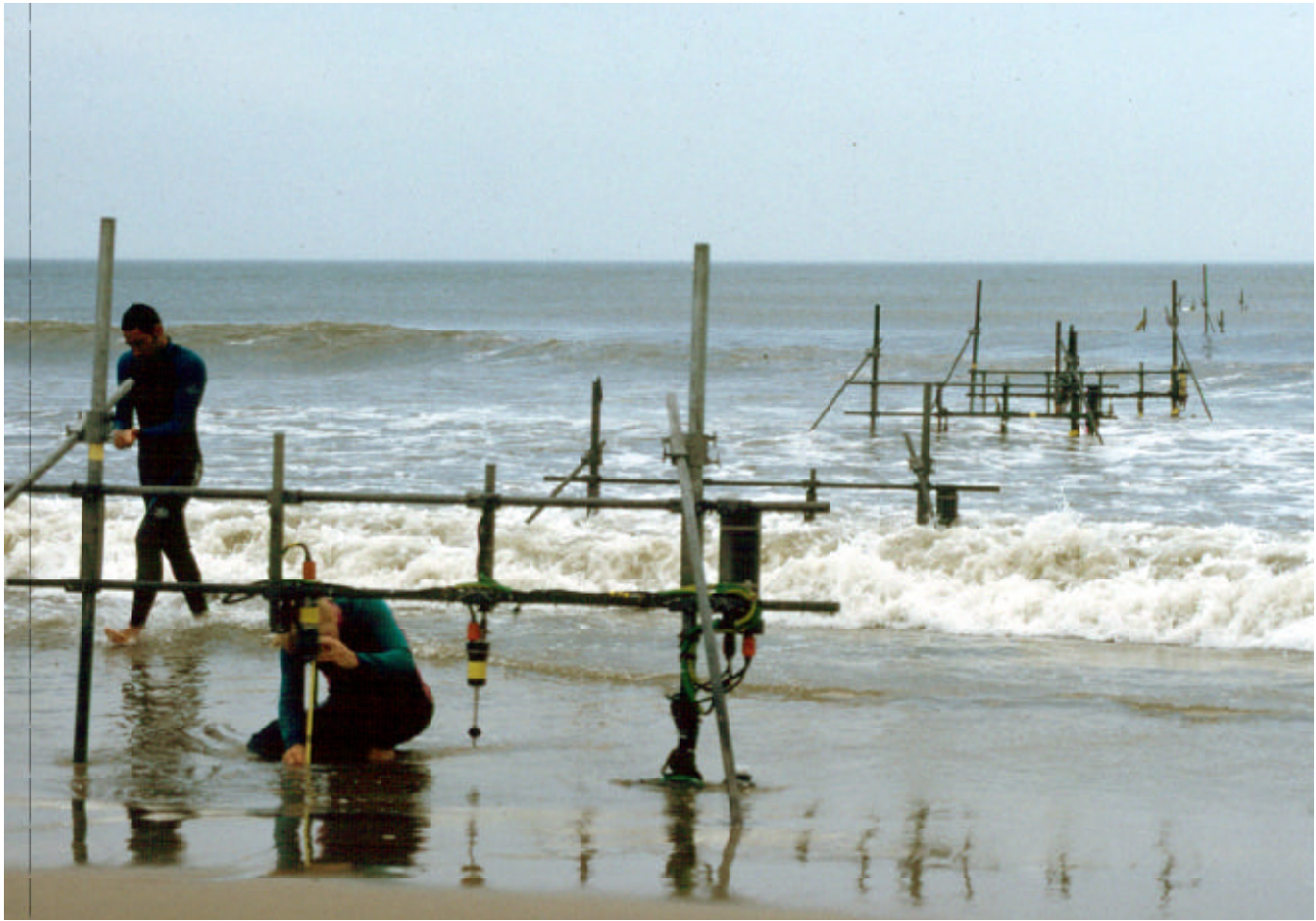
Figure 9. DUCK94 primary cross-shore instrument array being serviced. Unlike during DUCK85 (Figure 8), to provide continuous coverage even during storms, sediment-transport measurements during DUCK94 and SandyDuck were made with in situ instruments
