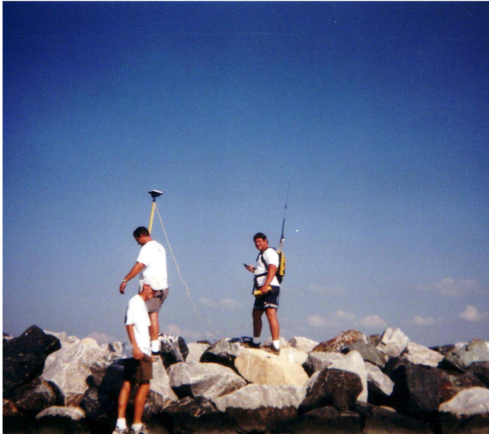
Figure 10. Jetty survey team using RTK-GPS gear with construction adhesive and paint as a marker point
