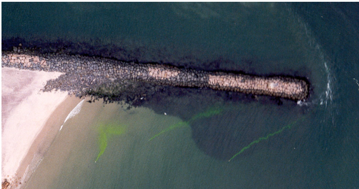
Figure 1. Dye release at Shinnecock Inlet (photograph courtesy of Aram Techunian, First Coastal Corp.)
