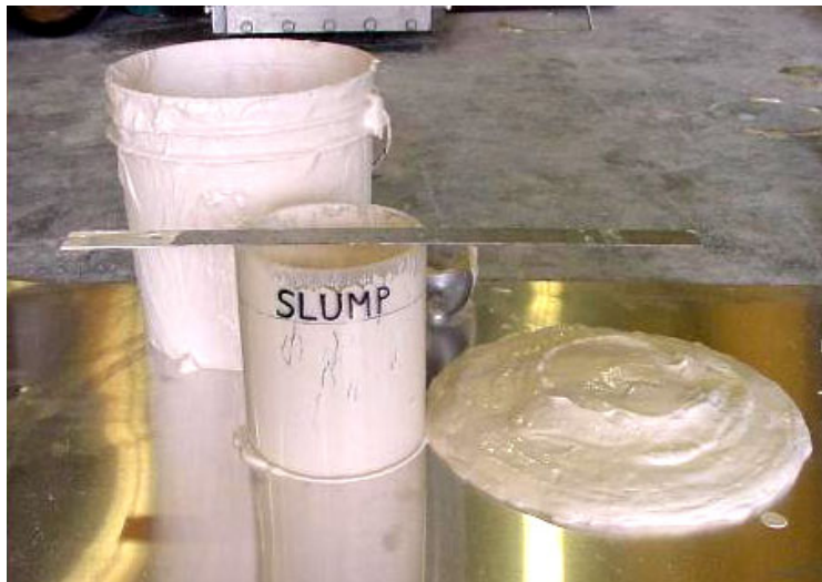
Figure 2. Slump test of kaolinite soil with approximate shear strength of 25 lbf/ft 2 (1.2 kPa)
