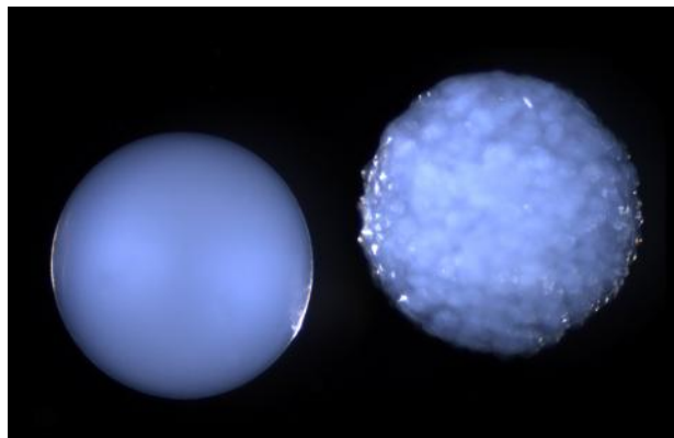
Figure 4. Alginate macro-spheres of 2 mm diameter. The sphere on the left is comprised of \text{Ca}^{++} -crosslinked alginate only. On the right, a similar alginate sphere is filled with heparin-Sepharose microbeads with an average diameter of 90 microns.
