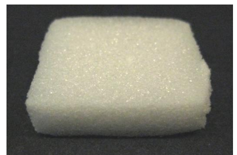
Figure 2. Example of a 0.75 mm thick, 8 mm diameter, disk-shaped gelatin sponge prototype perforated with an array of 0.4 mm diameter holes. The gelatin in this prototype was crosslinked with EDC/NHS.
