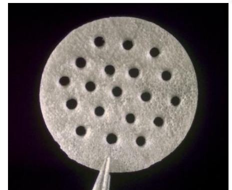
Figure 2. Example of a 0.75 mm thick, 8 mm diameter, disk-shaped gelatin sponge prototype perforated with an array of 0.4 mm diameter holes. The gelatin in this prototype was crosslinked with EDC/NHS.
