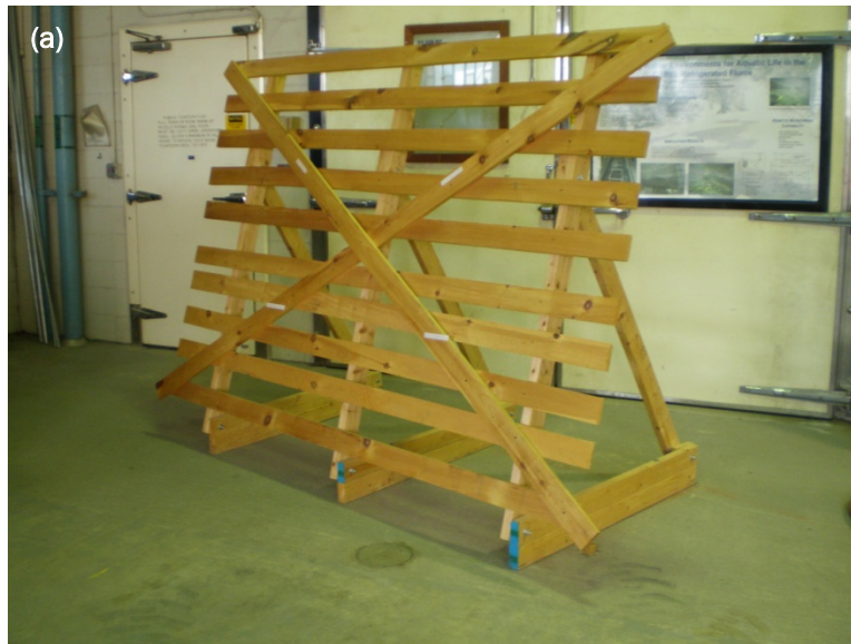
Figure 21. Wyoming snow fence (a) section and (b) installed on the Ross Ice Shelf, McMurdo, Antarctica.
