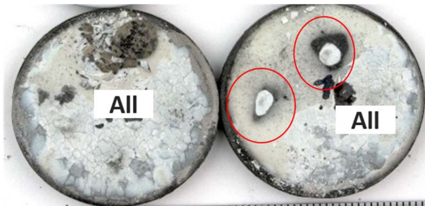
Figure 48: Button B illustrates missing TBC, indicated by the red circles, and in “All” regions.
