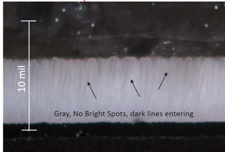
Figure 36: Optical cross-section of A1 and AFM sample heated to 1200 °C by dark field microscopy. A1 sample has a gradual boundary indicating where sample wet the surface. AFM sample presents colors typical of
