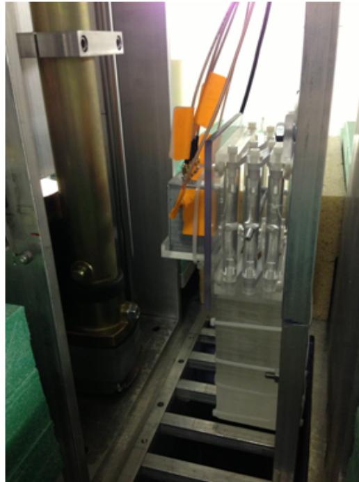
Figure 33. The test set-up inside the TMR included a block of acrylic to position the DuT fixture at the centerline of the beam. The acrylic jack sat atop this block. The aluminum test rig is positioned to the left of the jack and is facility the beryllium target (which is out of sight below and to the left of the set-up).
