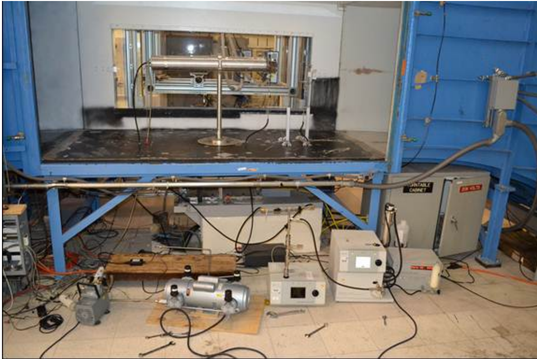
Figure A-17: Test Setup for Wind Tunnel Switch Testing
