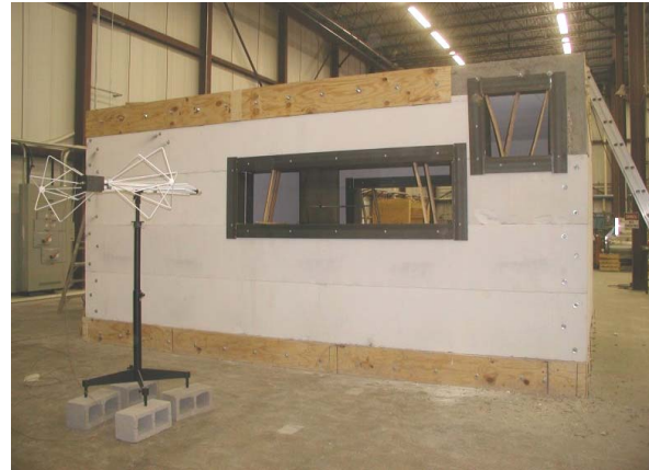
Figure 5: Explosive testing chamber and broadband receiving antenna
