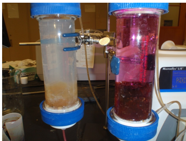
Figure 21. Photo showing the remaining colloidal silica matrix (left column) after \text{MnO}_4^- is released.
