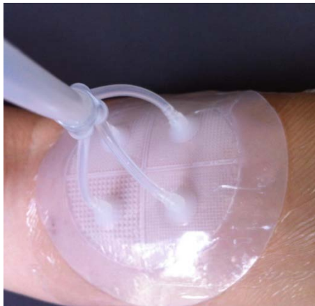
Figure 9: Fabricated device attached to human forearm (no wound).
