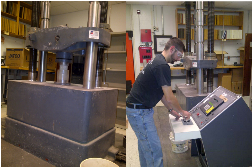
Figure 2. A 300K lb Riehle machine (shown above) was used to conduct all unconfined compressive strength testing.
