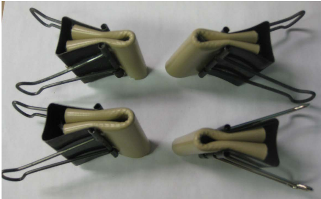
Figure 12. Specimens of bladder material double folded, clamped, and allowed to relax at room temperature.
