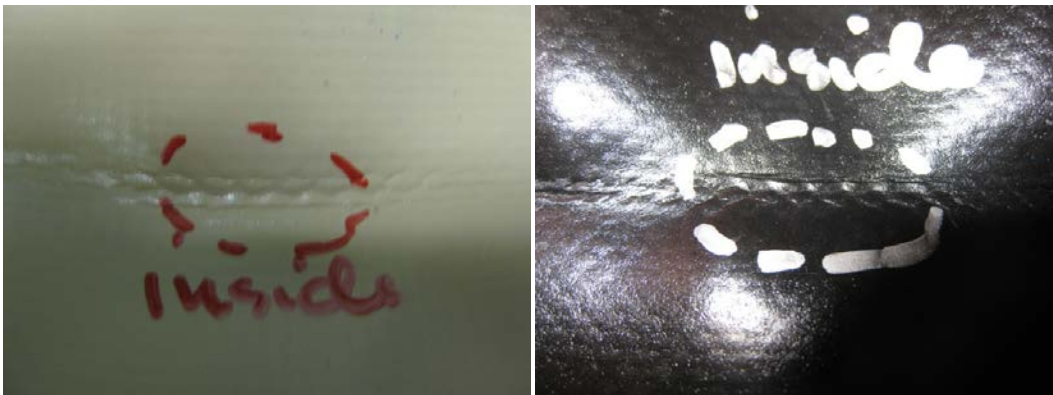
Figure 13. Bladder material creased but did not crack and leak at the inside corners of double folds when opened at -40^{\circ}\text{C} .
