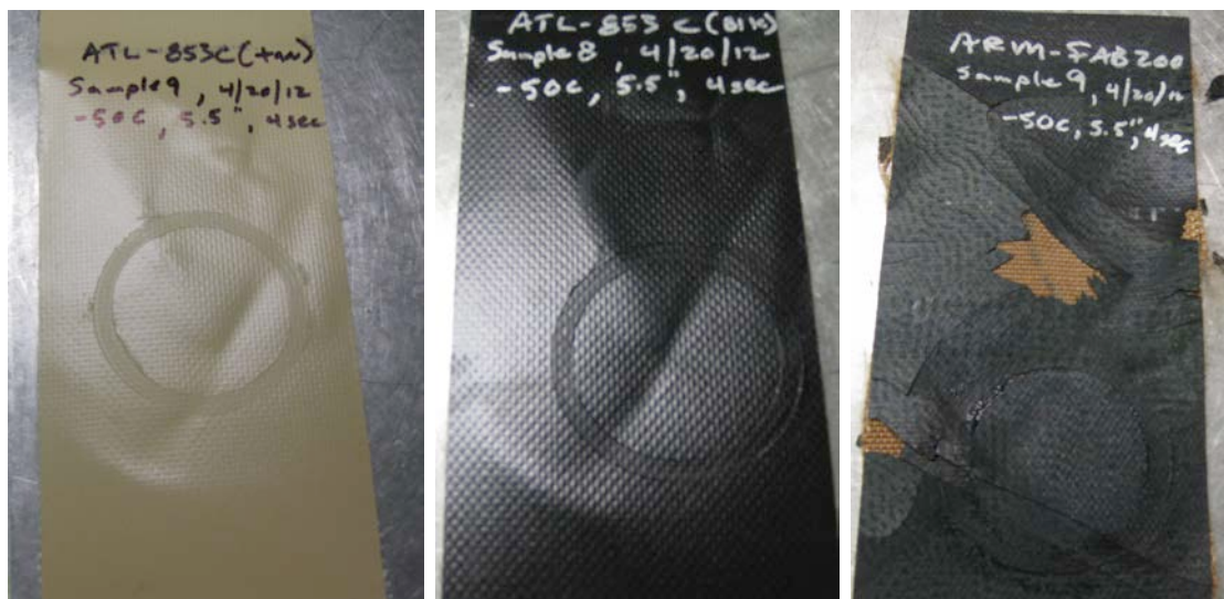
Figure 9. ARM-FAB200 specimens shattered and delaminated after one Gelbo cycle at -50^{\circ}\text{C} (right), while specimens of existing bladder materials (ATL-853C) survived 100 cycles at -50^{\circ}\text{C} without cracking and leaking (left and center).
