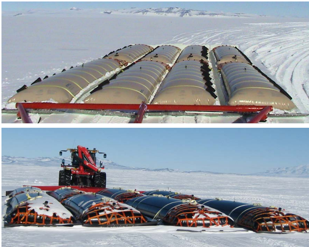
Figure 1. Fuel-bladder sleds ready for outbound transport on the South Pole Traverse from McMurdo Station to South Pole Station. The sleds consist of dual 3000 gal. fuel bladders strapped to 8 ft wide × 68 ft long × 0.5 in.-thick HMW-PE sheets towed through steel towplates. Sleds with black bladders produce lower sliding friction owing to solar gain, so SPoT is systematically replacing older tan bladders with black ones constructed from similar polyurethane-coated fabric.
