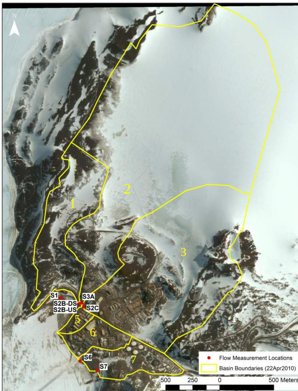
Figure 2. McMurdo Station watershed and sub-basin boundaries (Affleck et al. 2012a).
