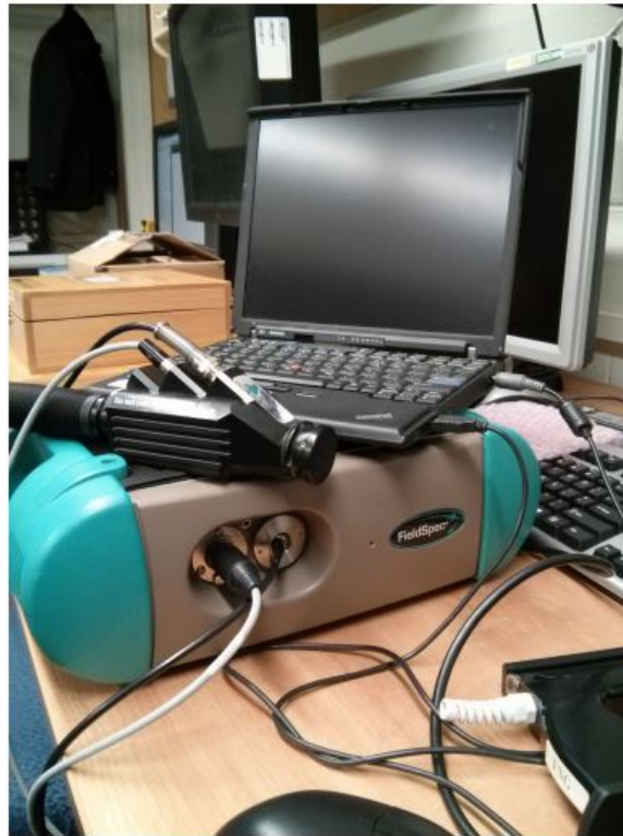
Figure 3.1: The ASD FieldSpec® 3 spectroradiometer attached to the ASD contact probe. The computer is for the software that controls the FieldSpec.
