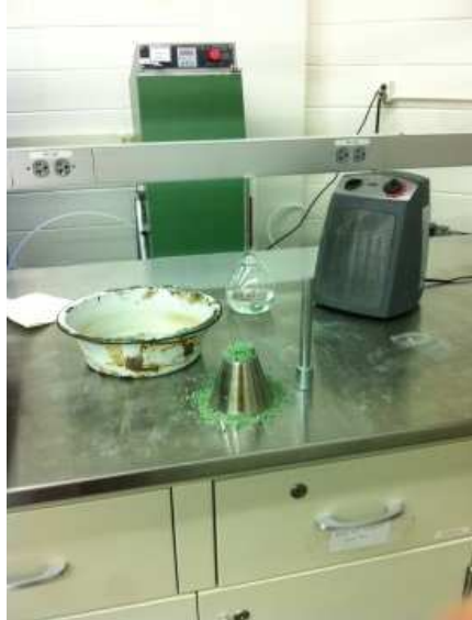
Figure 2 Surface Moisture Test to Determine Specific Gravity and Absorption
