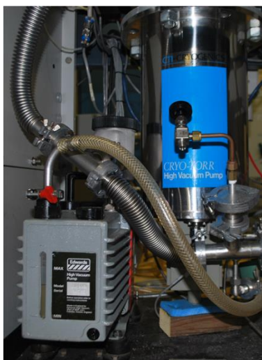
Figure 10 The Edwards (E2M28) high vacuum mechanical pump and the CTI Cryo-Torr 8 trapping pump.
