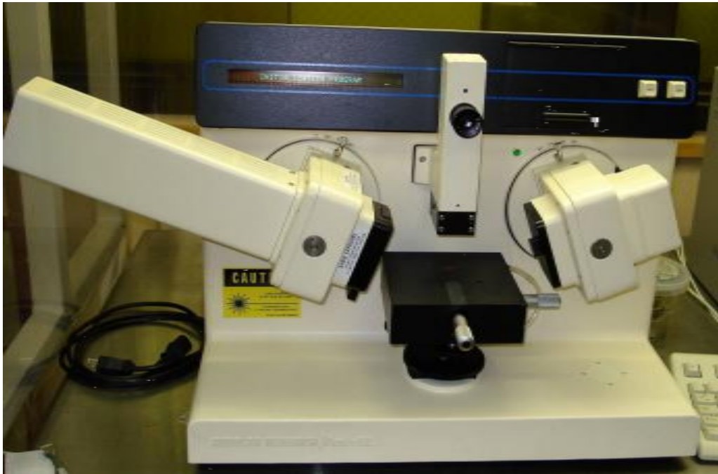
Figure 20 The Rudolph Research Auto EL II Ellipsometer used for film thickness analysis
