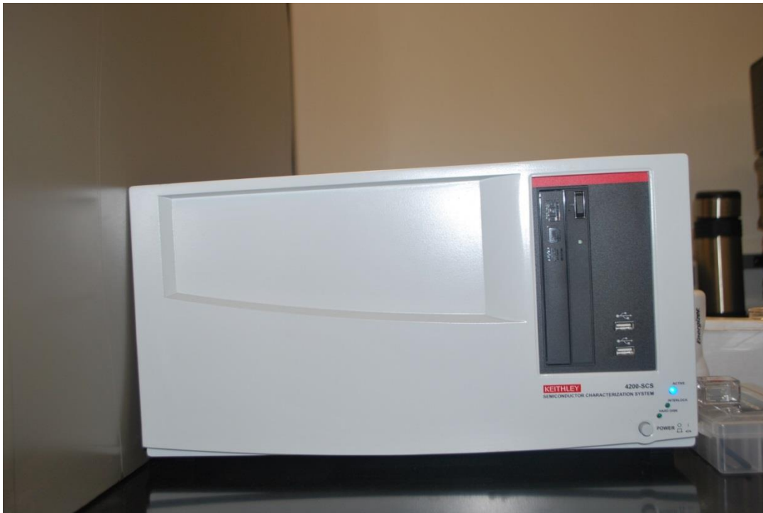
Figure 15 Keithley 4200 semiconductor characterization system used for I-V characterizations.
