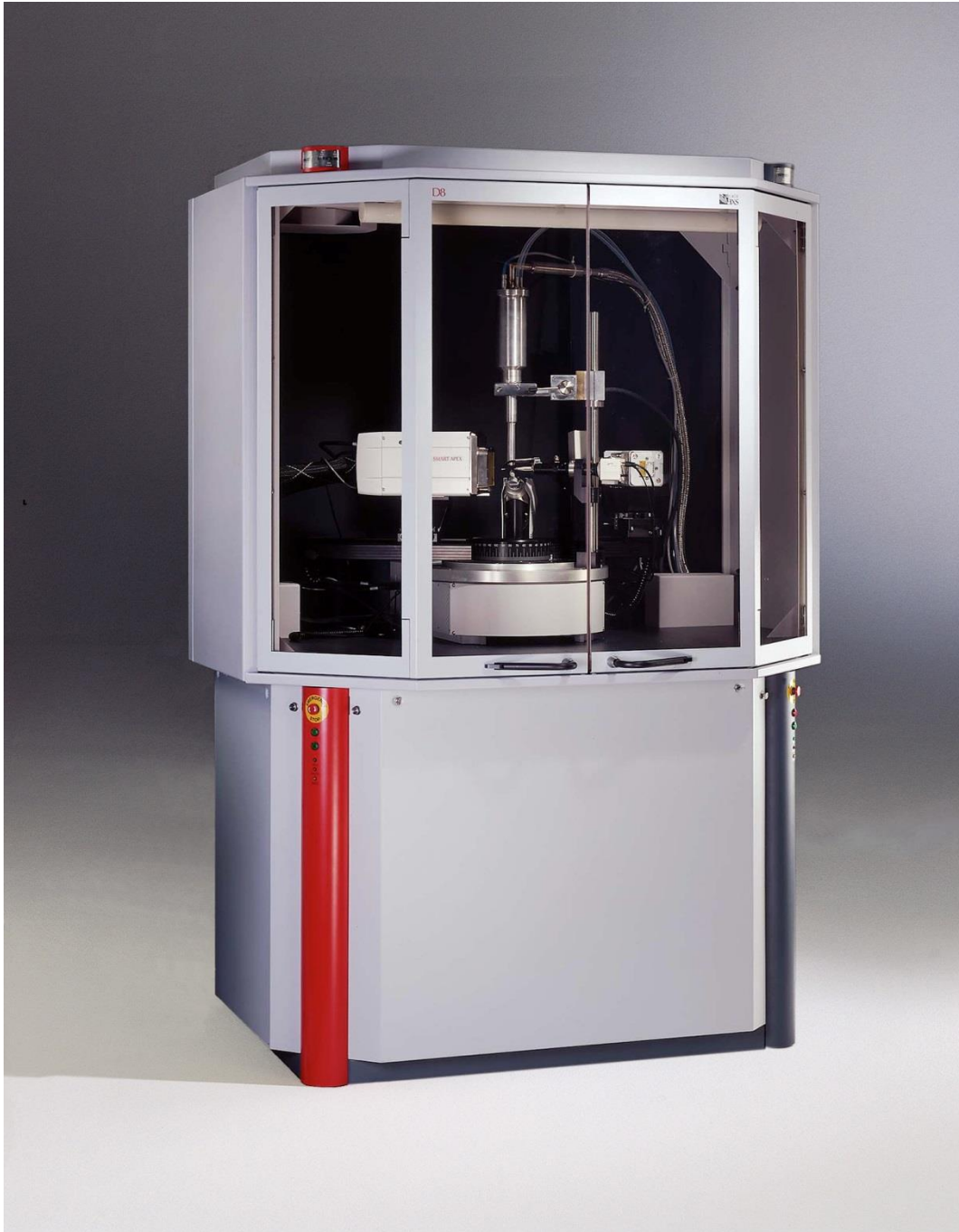
Figure 22 The Bruker AXS D9 Discover X-Ray diffractometer system used for XRR characterizations.
