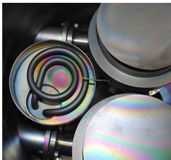
Figure 9 Radiant heater within the chamber of the Edwards ESM sputtering tool
