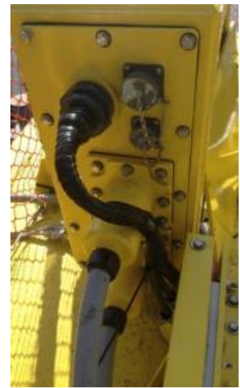
Figure 37: Junction box with watertight gland (Moran 2013).
