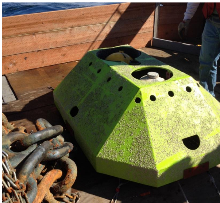
Figure 66: AWAC recovered on deck
