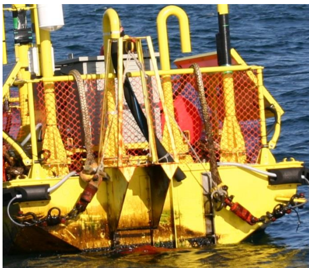
Figure 70: Load cells and swivels tied to bend restrictor (Hellin 2013-b)
