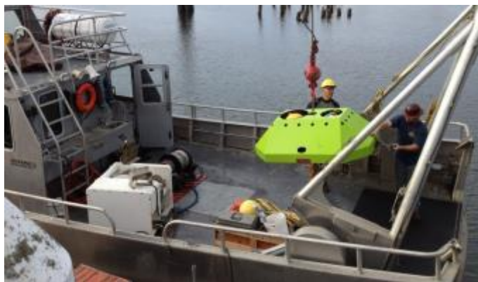
Figure 62: AWAC being loaded on R/V ELAKHA with Ship Ops Crane
