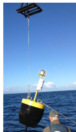
Figure 65: Corner marker buoy being lifted by boom
