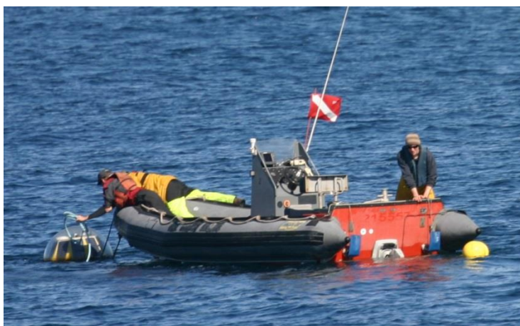
Figure 67: Recovery team attaching second lifting line to TRIAXYS (Hellin 2013-b)
