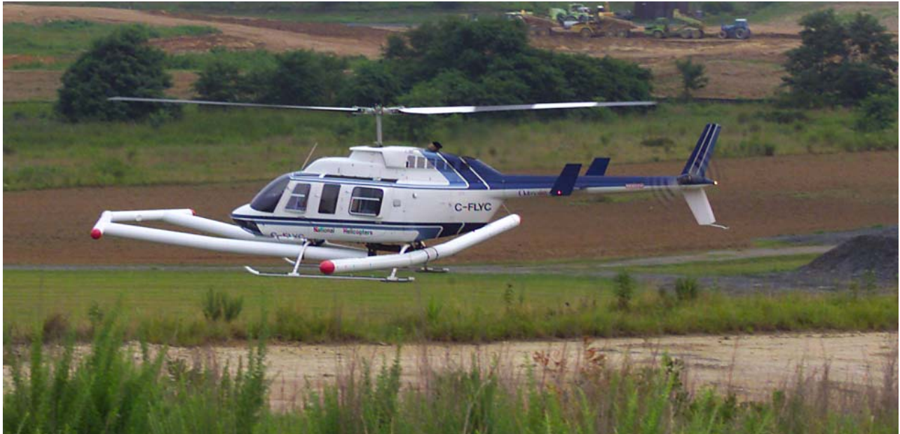
Figure 2.2 ORAGS-Arrowhead helicopter total field magnetometer system at APG (photo courtesy Gary Rowe, APG).
