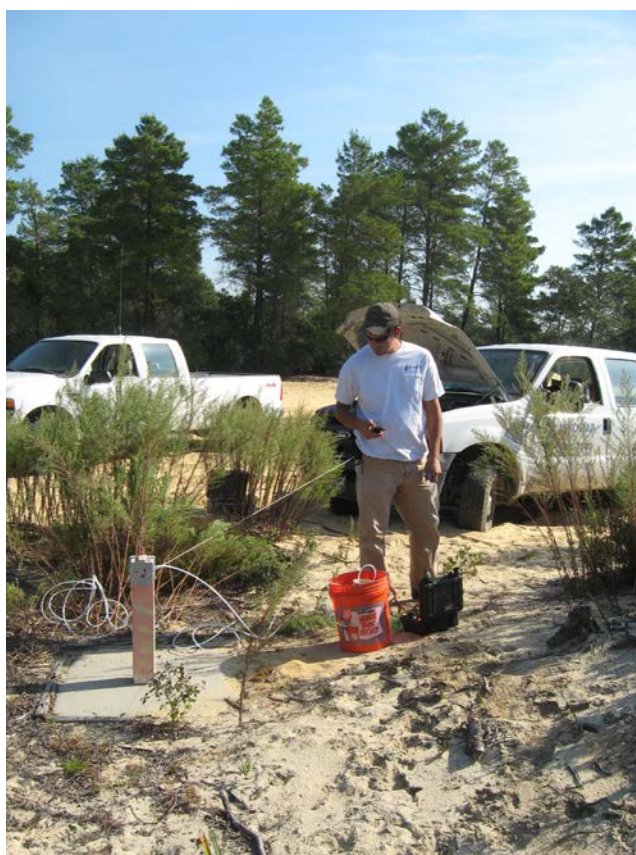
Figure 4-6. The well purging process.
