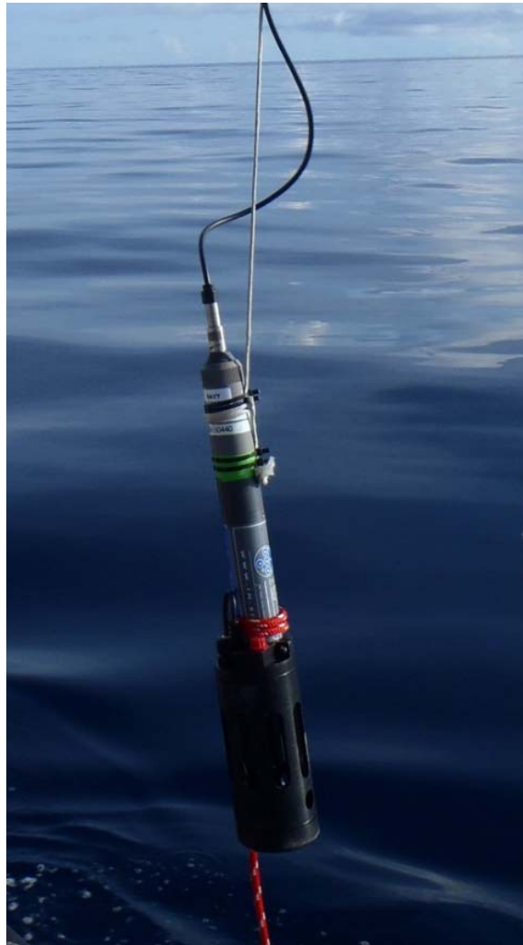
Figure 5. CTD unit ready for deployment.
