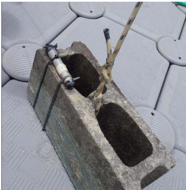
Figure 4. Levellogger® attached to concrete block ready for deployment.
