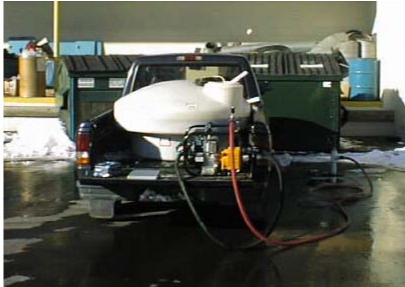
Figure 4-4. Vehicle Mounted Molasses Injection Rig
