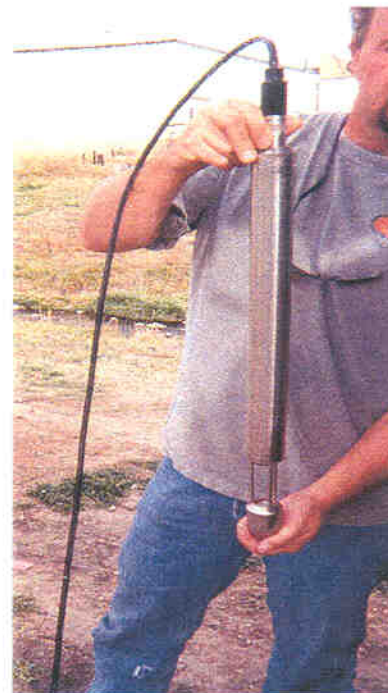
Figure 4-16. Colloidal borescope used at former Lowry AFB.
