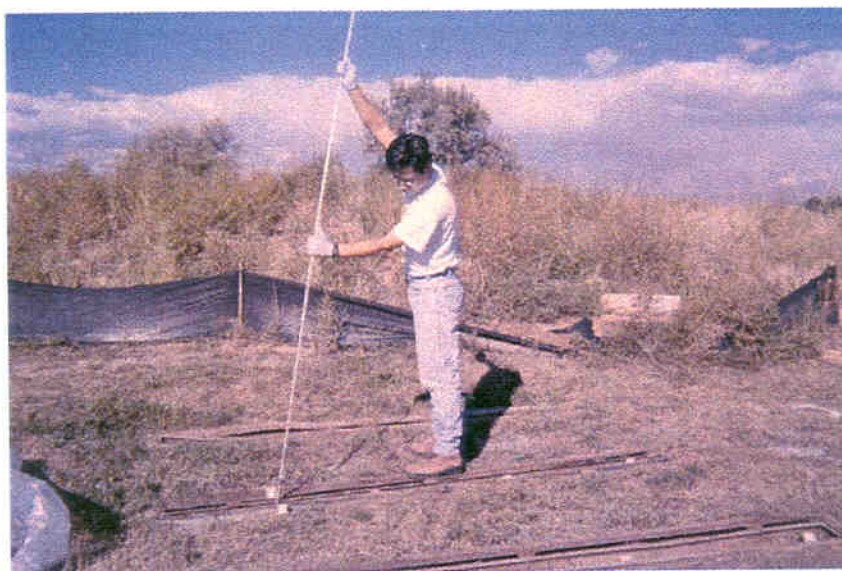
Figure 4-11. Collecting deposits from silt traps in monitoring wells at former Lowry AFB.
