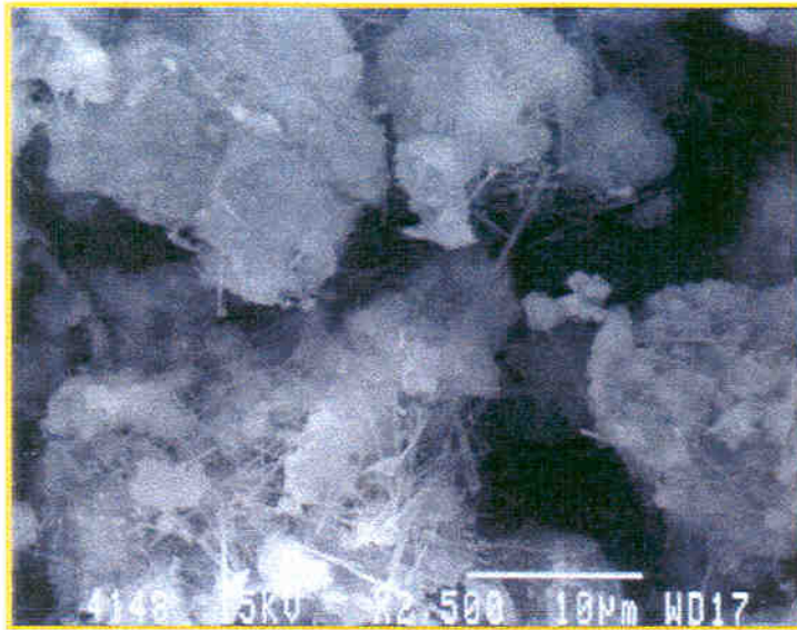
Figure 5-2. SEM micrograph of silt from well WW-12 showing Ettringite (needles) adjacent to calcite (plates).
