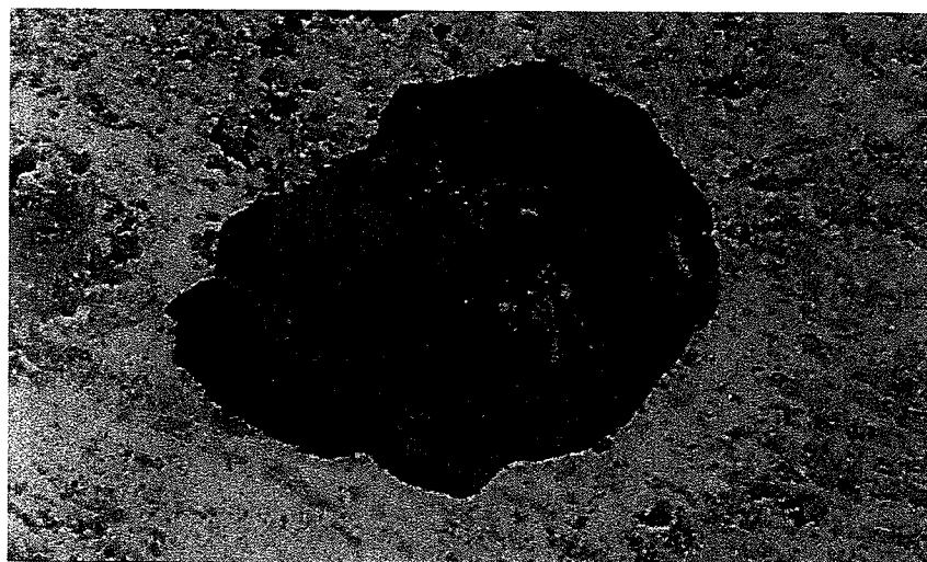
Figure 27. Low Order Detonation Residue on Soil Aggregate
