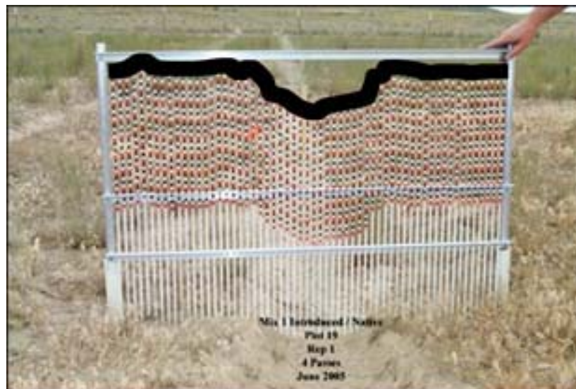
Figure 11. Pin profilometer used in a 4-pass rut immediately after tracking in June 2005.
