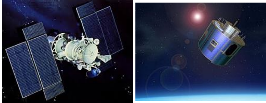
Figure 2.1: Box-wing type Gorizont (left) and cylindrical type Meteosat (right) satellite.
