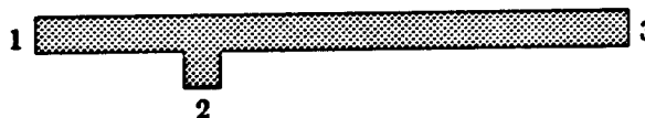
Figure 3.30: Resistance in multi-terminal nodes. Each node has a single resistance associated with it. When there are multiple connections to the node, any shorter paths (e.g. between 1 and 2) are billed the same amount of resistance as the longest path through the node (between 1 and 3).
